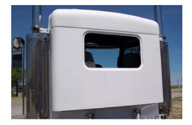
4. Fit day cab extension to cab, making certain in is centered side to side and top is flush with cab.
