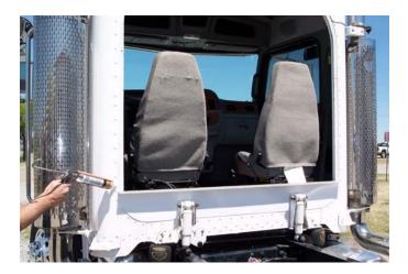
3. Run a continuous bead of adhesive sealer around entire edge of aluminum boot ring.
