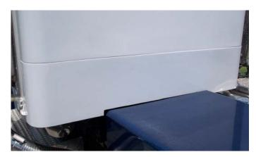
With air bags deflated fit lower skirt to cab, trimming may be required to allow min. ¼" clearance between frame and skirt. Bolt skirt from underside into rev-nuts using ¼"-20 bolts supplied.
