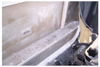
Run a bead of adhesive sealer around the interior edge of the filler panel, as well as the exterior edge. (Pictured in #8)
