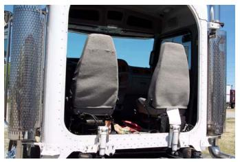
1. Remove existing air ride from sleeper and relocate to cab.
