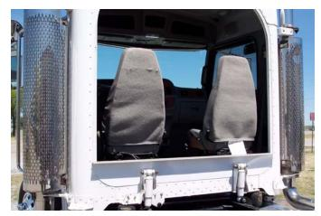
2. Place lower fiberglass filler panel Between shock towers and aluminum boot ring. (Do not fasten to cab at this time.)
