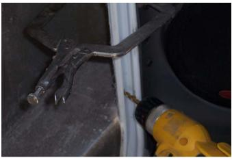
Starting at the bottom, drill holes through the aluminum boot ring and the fiberglass cab extension approximately 10-12 inches apart. Bolt together using the ¼ x 1" bolts supplied.
